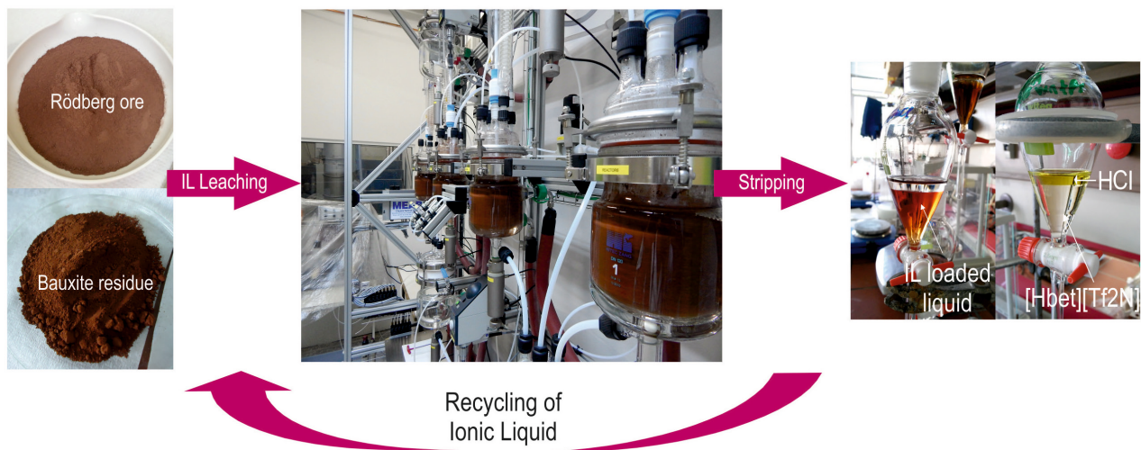
Figure 10 Ionic liquid leaching of Rödberg bastnäsite ore and red mud (or bauxite residue) (Balomenos et al., 2017). ©NTUA.
