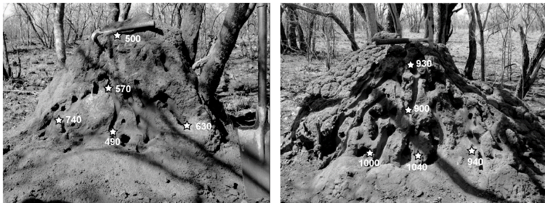
Figure 3: Y concentration (ppm) in termite mounds in the Blockspruit prospect in South Africa, measured by portable XRF analyser 14 .
